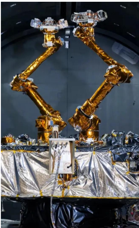
The DARPA Robotic Servicing of Geosynchronous Satellites (RSGS) payload, awaiting integration into Northrop Grumman's MRV.
