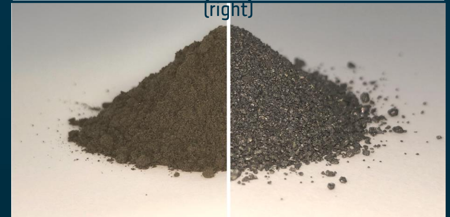
Regolith (left) and Oxygen extraction leftovers
